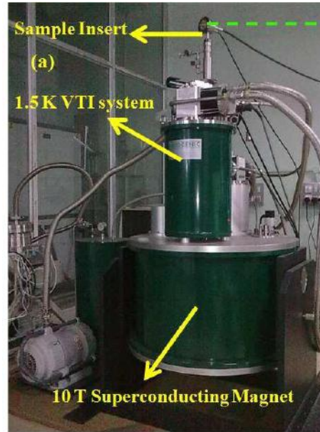
Figure 2.9: The picture of the 10 T magnet system from Cryogenic Limited used for magnetoresistance measurements. Image source Ref. [77].
